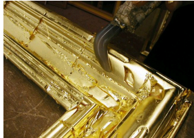
Smoothing of gold leaves with agate stone. Operation also called burnishing.
