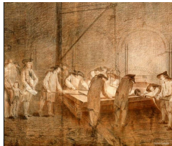
Casting of mercury mirror in Saint-Gobain with Pierre Delaunay-Deslandes, director of the manufacture from 1758 to 1789. Oil on canvas.
